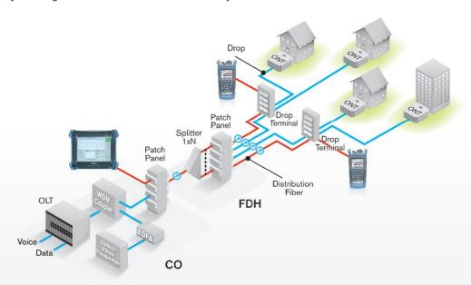
The FOT-930 allows for automated, bidirectional loss and ORL testing of passive optical networks (PONs) at 1310 nm, 1490 nm and 1550 nm, the three wavelengths recommended for PONs by ITU-T (G.983.3).
